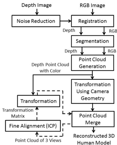
Figure 3: The architecture of the 3D Human Reconstruction System. The dotted arrows indicate an iterative flow.
