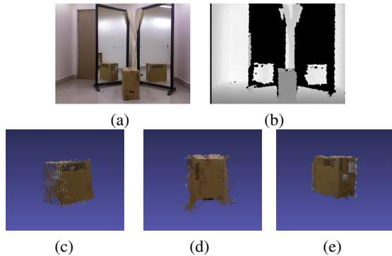
Figure 10: Experiment with a box object. (a) RGB view (b) Depth view (c) Reconstructed model viewed from right (d) From front (e) From left.
