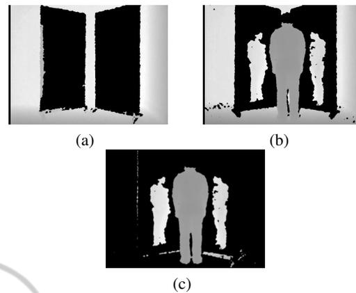
Figure 5: Noise Reduction. (a) Background depth image (b) Depth image with human (c) Difference depth image after noise reduction.
