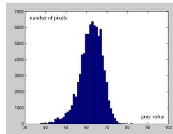
Figure 3: the histogram plot of biscuit without texture.
