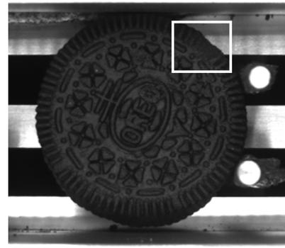
Figure 8: The result of partial fray biscuit.
