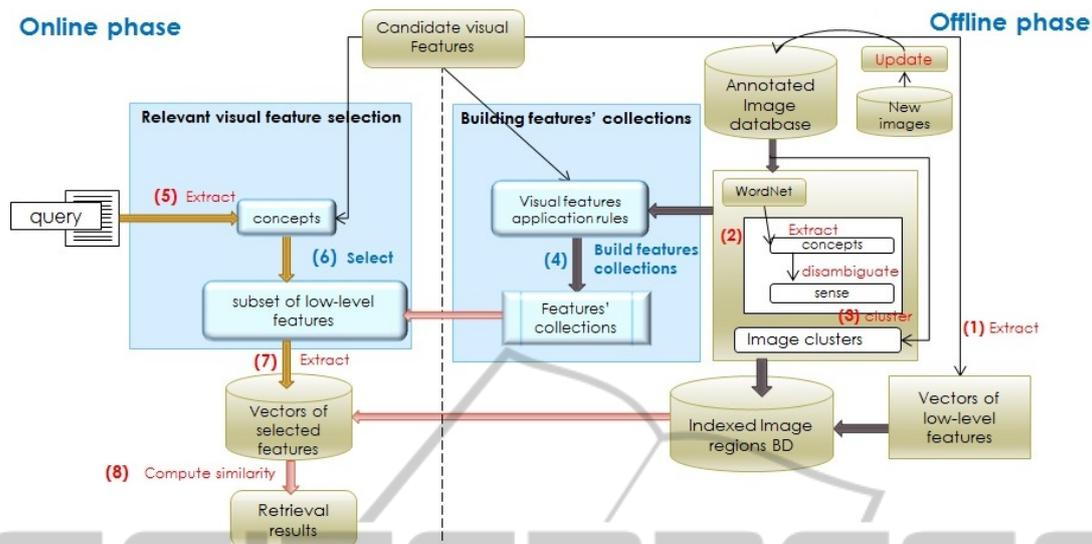
Figure 1: Relevant visual feature selection based approach.
