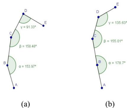
Figure 2: The sharp turn and zero curvature elimination. (a) sharp turn point is D, (b) zero curvature point is B.
