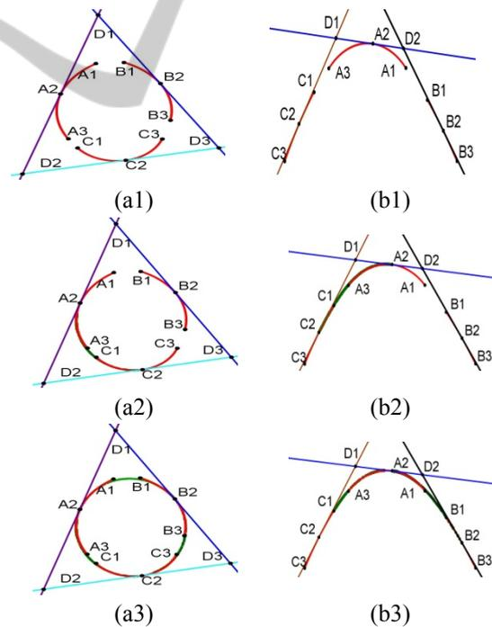
Figure 7: The procedure to merge the conic edge segments as a part of an ellipse (a1-a3) and a parabola (b1-b3).
