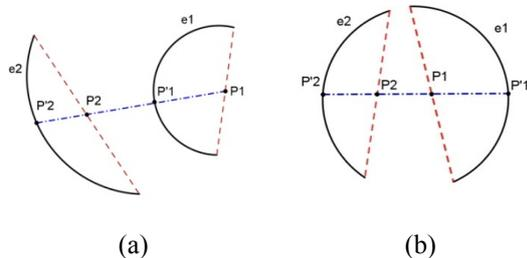
Figure 6: The condition of associated convexity (a)  $e_1$  and  $e_2$  cannot be grouped together, (b)  $e_1$  and  $e_2$  can be grouped together.
