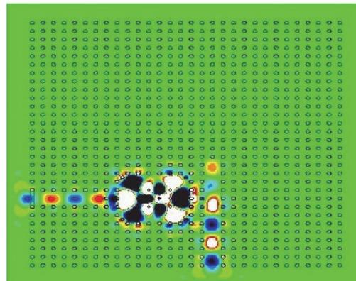
Figure 6: The steady mode field distribution when the incident wavelength is  $83.535\mu\text{m}$ .
