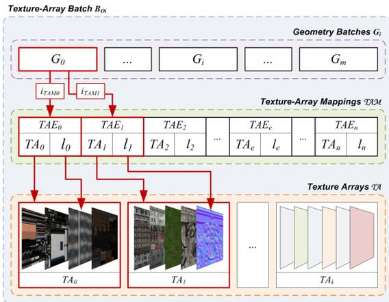
Figure 4: Concept for sampling texture arrays  $\mathcal{TA}$  at runtime. Each geometry batch  $G_i$  can reference one or more array mapping entries  $TAE_e$  within the texture array mapping  $\mathcal{TAM}$ . These entries refer to a bound texture array  $TA_e \in \mathcal{TA}$  and the respective layer  $l_e$  to sample from (see Listing 1 for an exemplary GLSL implementation).
