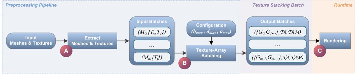
Figure 3: Overview of the pre-processing and rendering pipeline for the presented batching approach. In an off-line processing step the input geometries and texture data are sorted (A) before the actual batching process is performed (B). The batching process delivers a number of texture arrays, geometry batches, and texture array mappings, which are rendered by using shader programs (C).
