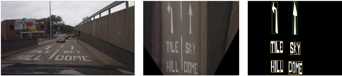
Figure 3: Stages of MSER detection on IPM image, showing original frame (left), IPM image (centre), and detected MSERs, with detected words marked in orange and symbols in green (right).
