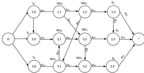
Figure 2: Oriented disjunctive graph of the SC of Figure 1.
