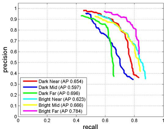
Figure 6: The performance of head-shoulder DPM model (trained using around 9000 positive images, cascade PCA 5, the overlap area > 50%).
