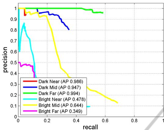
Figure 5: The performance of the full body ACF detector (trained using the Inria dataset, the overlap area > 10%).
