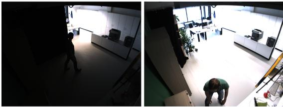
Figure 8: The left and right images are the samples in the test group of dark-mid and bright-near respectively.
