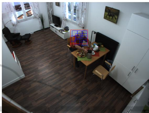
Figure 3: Exemplary detection of the DPM algorithm using the proposed head-shoulder model. When using the head-shoulder model, the person sitting at the table can be detected.
