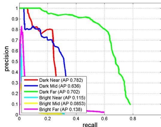
Figure 7: The performance of head-shoulder ACF detector (trained using around 9000 positive images, the overlap area > 50%).
