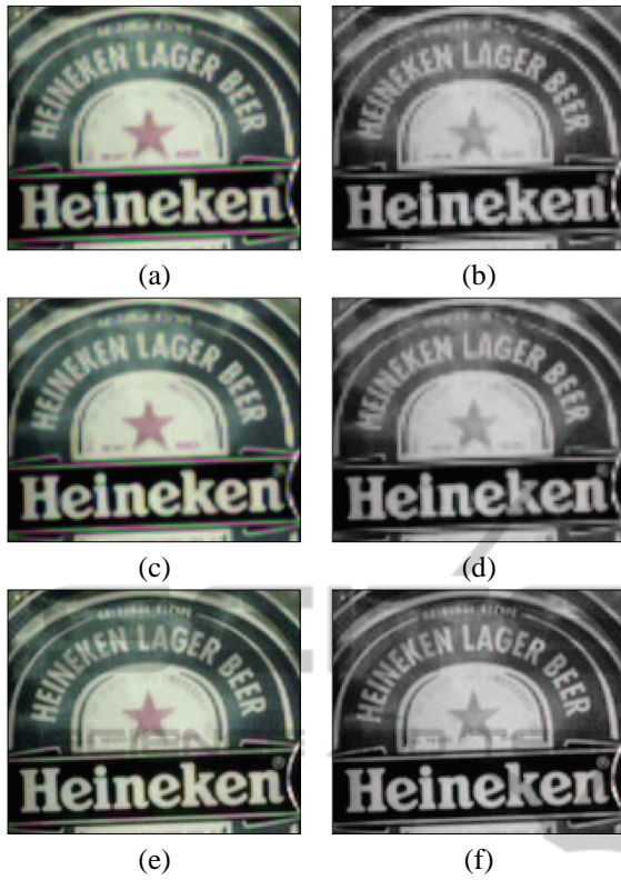
Figure 8: Part of the Sample4 image. (a) Color result of the bilinear interpolation. (b) Color result of the BTES method. (c) Color result of the proposed algorithm. (d) NIR result of the bilinear interpolation. (e) NIR result of the BTES method. (f) NIR result of the proposed algorithm.
