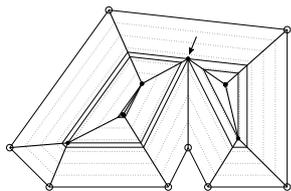
Figure 3: An example of straight offset polygons.
