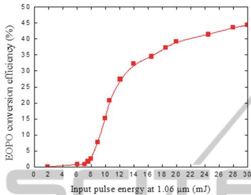
Figure 7: EPO conversion efficiency as a function of the input pulse energy at 1.06 μm.
