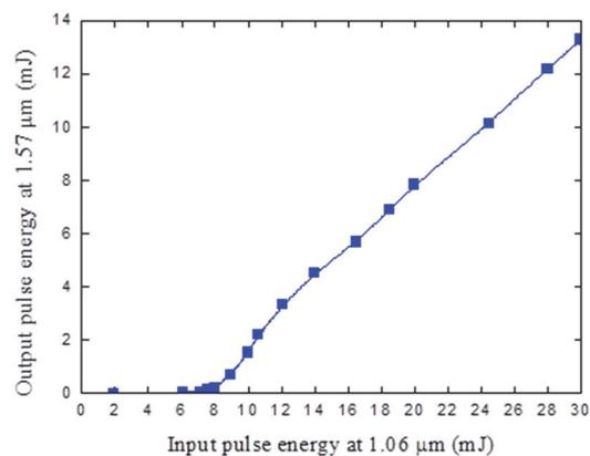
Figure 6: Output pulse energy at 1.57  $\mu\text{m}$  as a function of the input pulse energy at 1.06  $\mu\text{m}$ .
