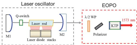
Figure 1: Experimental configuration for an extracavity OPO with a monolithic KTP crystal pumped by the passively Q-switched Nd:YAG/Cr<sup>4+</sup>:YAG laser oscillator with a convex-concave resonator.
