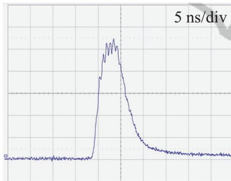
Figure 8: Temporal behavior of the OPO pulse at 1.57 μm.
