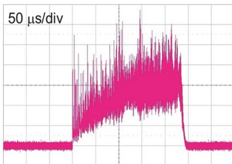
Figure 3: Temporal shape for the laser pulse at the maximum diode pump energy of 298 mJ.
