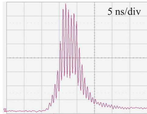
Figure 4: Temporal shape for the 1064-nm laser pulse.
