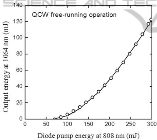
Figure 2: Output energy at 1064 nm with respect to the diode pump energy at 808 nm in the QCW free-running operation.
