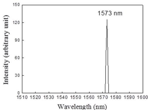
Figure 9: Optical spectrum measurement for the OPO.
