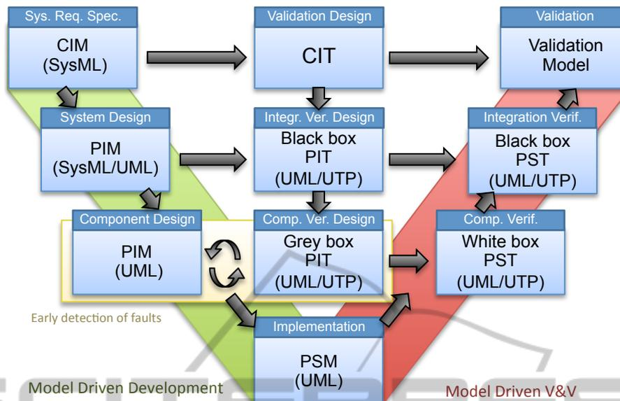
Figure 2: The proposed model-driven V-Model. Boxes show the activities, the models produced, and the formalisms used. The arrows represent dependency between artifacts. The *Component Design* has a dependency with the *Component Verification Design* if it exploits the test model to early detect faults.
