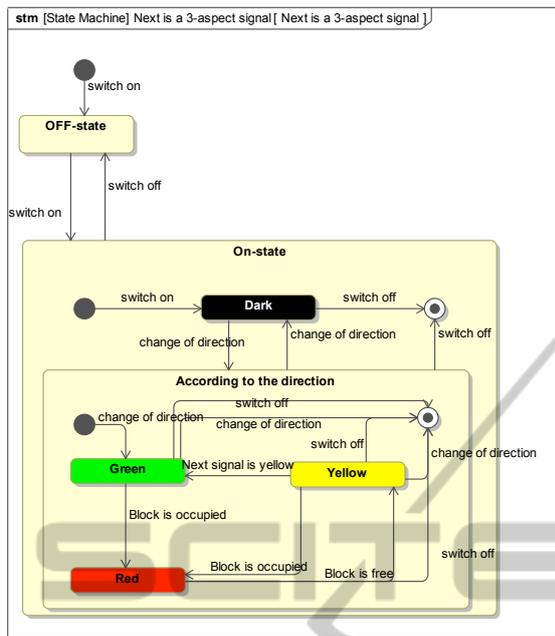
Figure 3: CIM state diagram showing the required dynamic behavior of three lights semaphore.
