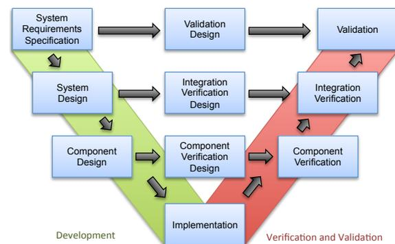
Figure 1: A V-Model process.
