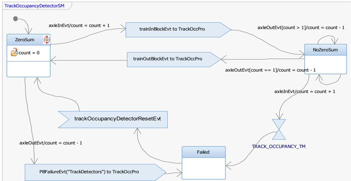
Figure 5: The PIM diagram representing the behavior of the TrackOccupancyDetector.
