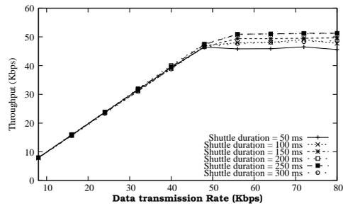
Figure 8: Throughput comparison by Shuttle duration in a 3-Redundant LSN.
