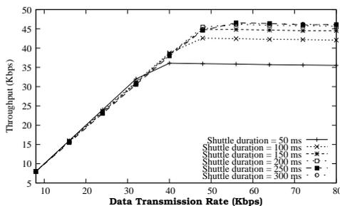
Figure 7: Throughput comparison by Shuttle duration in a 2-Redundant LSN.
