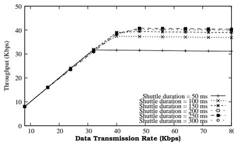
Figure 6: Throughput comparison by Shuttle duration in a 1-Redundant LSN.
