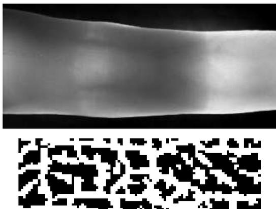
Figure 1: Finger vein from Twente database and its corresponding balanced coding.
