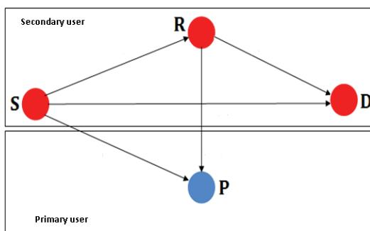
Figure 2: Relay Technique with Underlay Cognitive Radio Technology.
