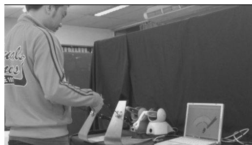
Figure 1: Physical interface, of BART LAB's VR training system, which attaches laparoscopic tools to two Phantom Omnis; haptic devices used for user interaction.
