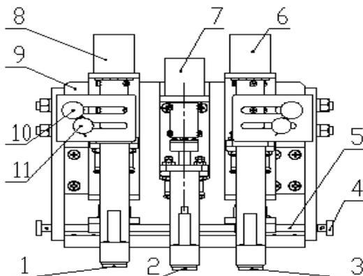
1—sensor of Chi region 2—sensor of Guan region 3—sensor of Cun region 4—x-axis position adjustment knob 5—x-axis threaded shaft 6—pressure controlling module of Cun 7—pressure controlling module of Guan region 8—pressure controlling module of Chi region 9—fixed bracket 10—y-axis fixed knob 11—y-axis position adjustment knob
