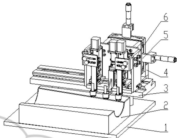
1—base 2—wrist bracket 3—sliding guide table 4—connecting plate 5—x-y axes precise manual adjustment platform 6—three-probe pulse sensor
