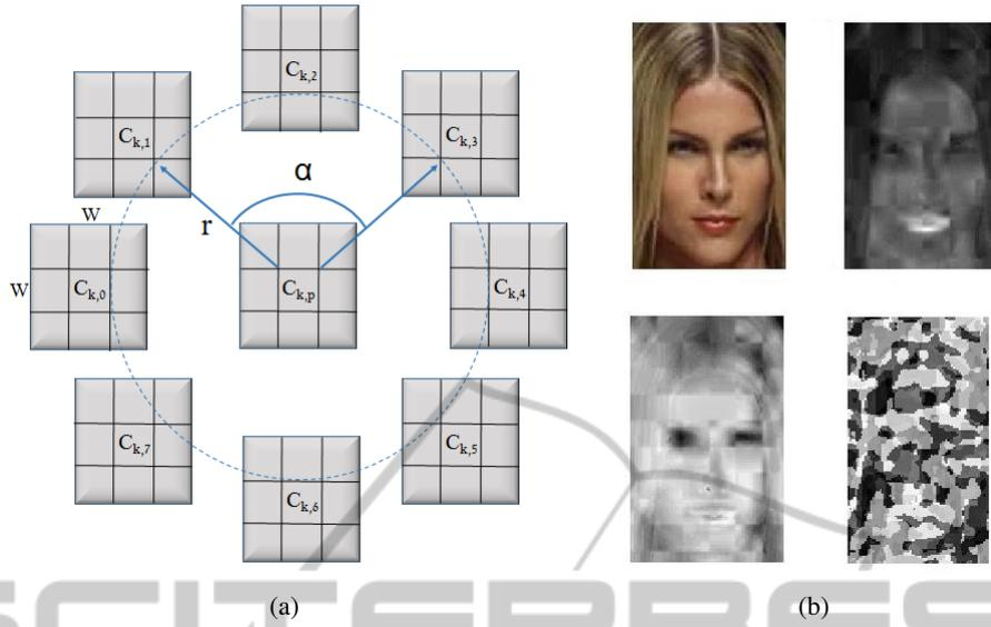
Figure 1: CC-TPLBP code computation. (a) CC-TPLBP operator for a single chroma channel, with parameters  $\alpha = 2$ ,  $S=8$  and  $w=3$ . (b) An example of CC-TPLBP code for a color face image. Upper left - face image; upper right - CIE-Lab  $a$  chroma; lower left - CIE-Lab  $b$  chroma ( $a$  and  $b$  are presented as gray-level images); lower right - CC-TPLBP code image. The parameters used are  $r=5$ ,  $S=8$ ,  $w=4$ .
