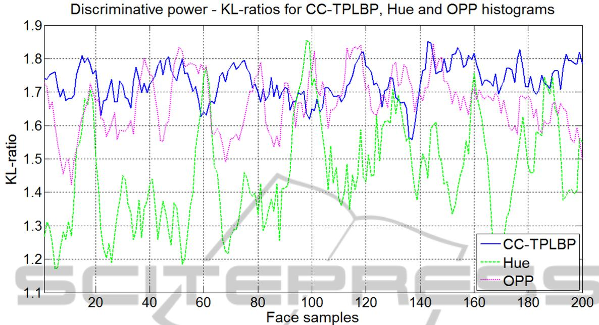
Figure 3: Discriminative power measure. KL-ratios of 200 face images with 200 background images. Horizontal axis: face sample numbers; vertical axis: KL-ratio values computed by Eq. (7). The displayed KL-ratios are smoothed using a uniform averaging filter of size 7, for further explanation see text. It can be seen that CC-TPLBP (blue curve) has the highest mean KL-ratio and lowest variance, as also seen in Table 3.
