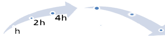
Fig. 4. MultiGrid scheme. The fine level ( h ) is transferred to the coarser level ( 2h ), and then recursively until the coarsest level is reached. Then backwards the solution is transferred to the finer level etc. until the finest level is reached again.
