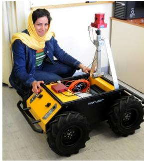
Figure 5: The bio-inspired autonomous robot implements target detection algorithms derived from electrophysiological recordings.
