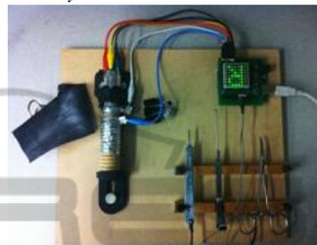
(b) Six different landmarks represented by conductive foils and tools (scalpel, hook and forceps) are connected to microcontroller for data collection.
