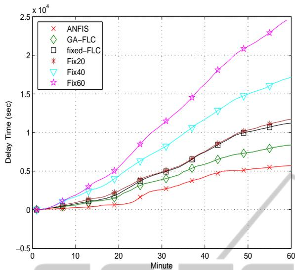
Figure 7: Accumulative total delay time of the intersection in one hour.
