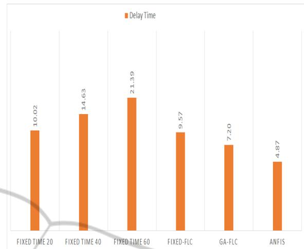
Figure 8: Total delay time per vehicle for the intersection.
