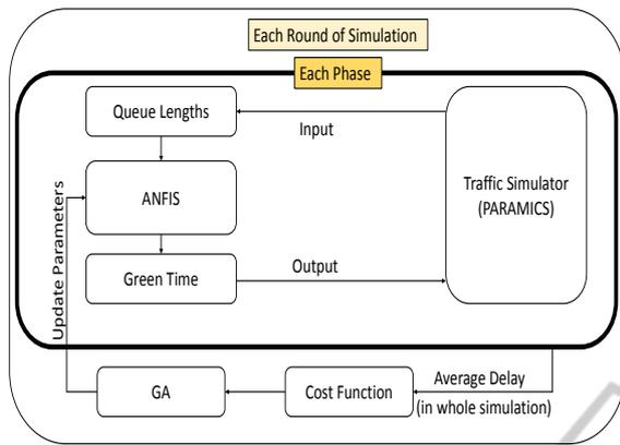
Figure 1: The figure shows the process of ANFIS training. ANFIS parameters are updated after each round of simulation through genetic algorithm optimization method.
