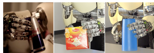
Figure 6: Grasping a variety of objects successfully, such as, tin cans, plastic cups and tea boxes. The module works for both the right and left hand.
