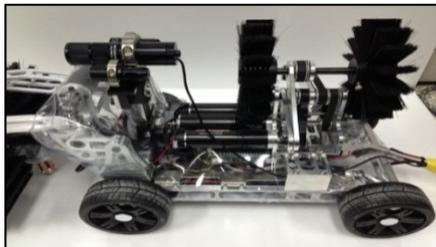
Figure 7: Prototype of the duct cleaning robot.
