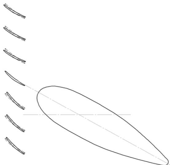
Figure 4: Rotation scheme of guide vane blades.
