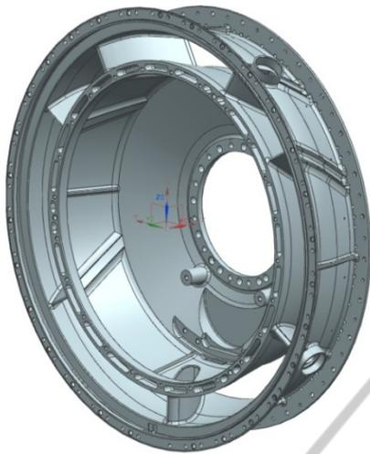
Figure 2: Casing of middle support.
