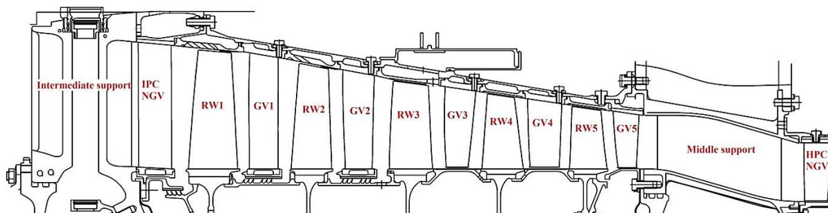
Figure 1: The scheme of investigated compressor blading.
