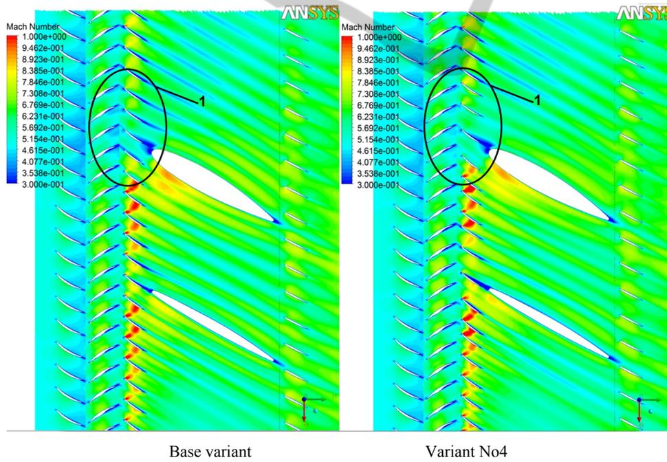
Figure 7: Mach number field close to lower support rack.
