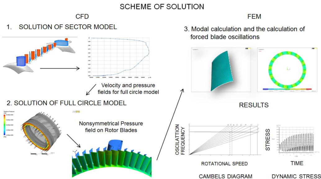
Figure 3: The scheme of method for calculation compressor rotor blades forced oscillations.
