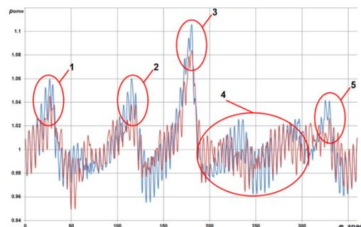
Figure 5: Relative static pressure variation in the section following the IPC RW5 at mid-span.
