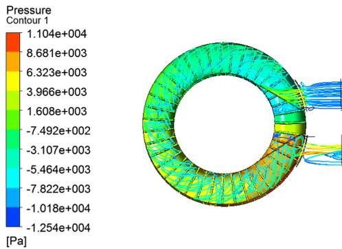
Figure 9: Streamline and static pressure of newly designed blower.
