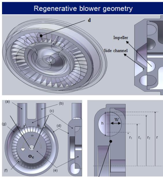
Figure 1: Geometry and design variables of regenerative blower.
