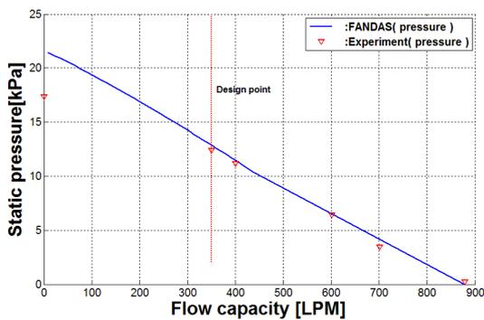
Figure 11: Pressure curve of newly designed blower.
