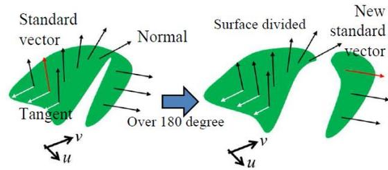
Figure 3: Condition of divided curved surface.
