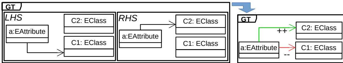
Figure 1: A graph transformation rule shown as divided view and merged view.
