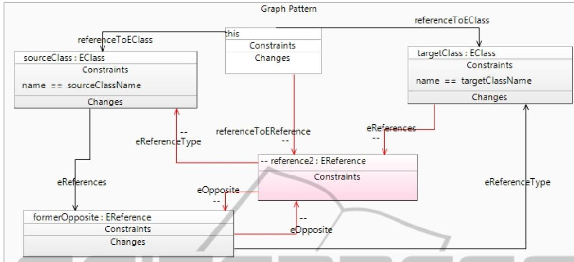
Figure 4: Rule for changing a bi- to a unidirectional reference in an Ecore class diagram.
