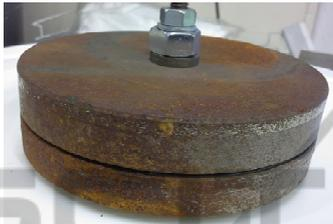
Figure 3: Surface corrosion of metal discs.
