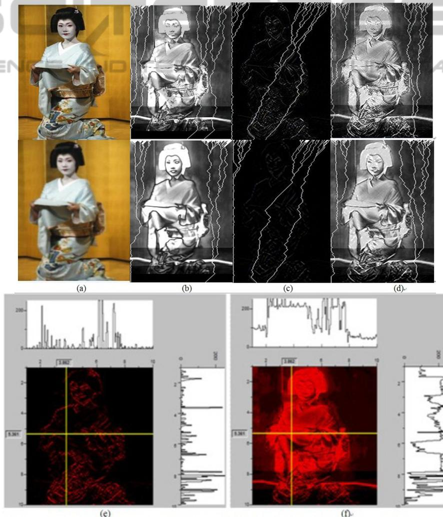
Figure 5: Column (a) shows original (above and noise version (below) of the image. Column (b)(c)(d) shows several less energy stitching lines calculated on prominence map, gradient map, improved energy map. (e) and (f) are profiles of gradient map and improved energy map respectively.
