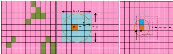
Figure 4: (a) Tentative detection based on global contrast. (b) The prominence detection based on local contrast of an image region with respect to its neighborhood is defined within a circle of radius  $r$ . (c) Filtering the images at one of the scales in rotate-expanding manner.
