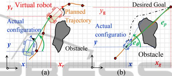
Figure 2: (a) Trajectory tracking problem based on virtual approach, (b) reactive navigation problem in unknown environment.
