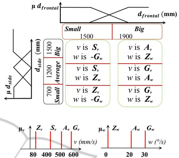
Figure 6: Fuzzy rules basis and outputs sets for the obstacles avoidance controller.
