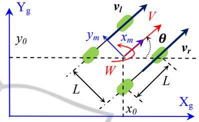
Figure 1: Kinematics of the Pioneer P3-AT mobile robot.
