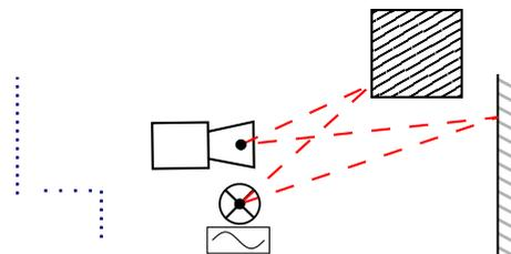
Figure 1: Idealistic Sensor Model. The LED emits modulated light which is reflected by the scene on the right (dashed red paths). From the phase-offset of the received light the sensor can calculate distances and these can be used to build a 3D model of the scene (blue dots on the left). The wave length of the modulation is ideally greater than the longest path lengths expected in the application.
