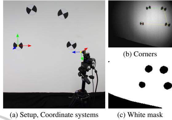
Figure 6: White wall with markers. We covered the floor with low-reflective textile to limit multi-path reflections.
