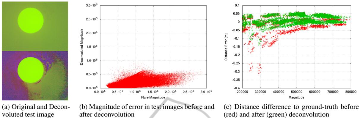
Figure 8: Figures (a) and (b) show the results of deconvoluting the training images. Figure (c) shows the difference to a checkerboard ground-truth distance, before and after compensating the scattering effect dependent on the magnitude of received light.
