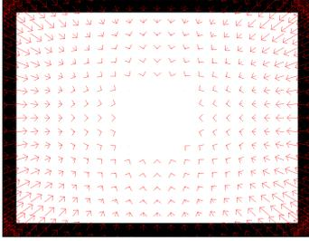
Figure 4: Lens Distortion. The arrows point from the theoretical undistorted point to the distorted point. Distortions below 1 px are not shown. The image border is marked black. As common for wide-angle lenses the distortion near the borders is very high.
