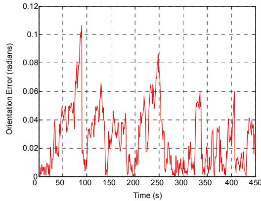
Figure 7: Orientation error for UKF mapping without data association scheduling for  $v=1\text{m/s}$ .
