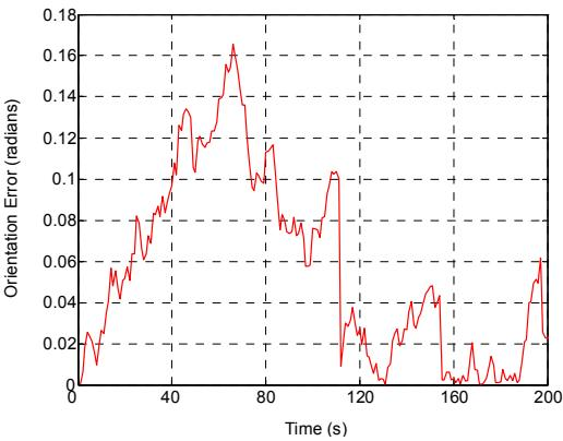
Figure 11: Orientation error for UKF mapping without data association scheduling for  $v=5\text{m/s}$ .
