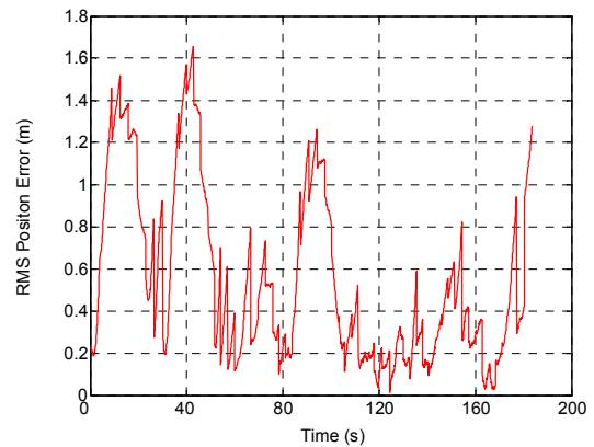
Figure 9: RMS position error for UKF mapping without data association scheduling for  $v=5\text{m/s}$ .
