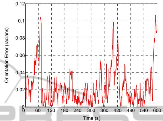
Figure 8: Orientation error for UKF mapping with data association scheduling for  $v=1\text{m/s}$ .
