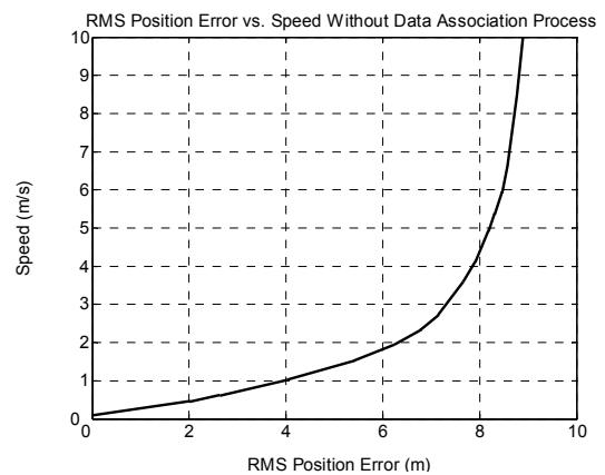
Figure 13: RMS position error for global map estimation without data association technique for  $v=1\text{m/s}$  to  $10\text{m/s}$ .
