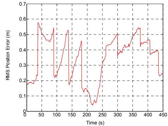
Figure 5: RMS position error for UKF mapping without data association scheduling for  $v=1\text{m/s}$ .
