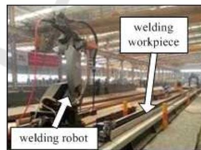
Figure 2: Welding robot in crane welding production line (Provided by Nucleon (Xinxiang) Crane Co., Ltd in Henan, China).
