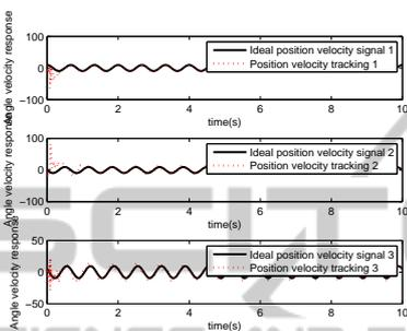
Figure 6: Ideal position velocity signal and position velocity tracking output.
