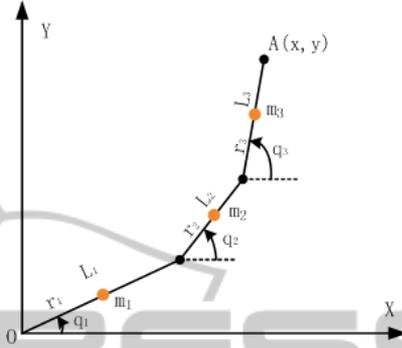
Figure 3: A 3-link robot manipulator.
