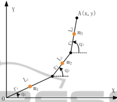
Figure 3: A 3-link robot manipulator.
