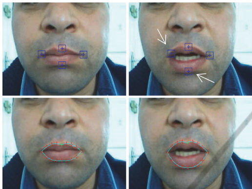
Figure 12: Tracking of lip movement: (a) (b) followed by vote algorithm of (Mahdi, 2008), (c) (d) followed by our method (filter particles).
