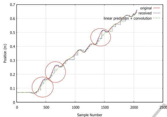
Figure 10: Restoration results when the maximum velocity is less than the original one. At several places enclosed by red circles, the green line cannot follow the red line because of the hardware limits.
