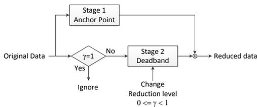
Figure 1: Flow chart for data reduction: The original data is reduced by two-stage process.
