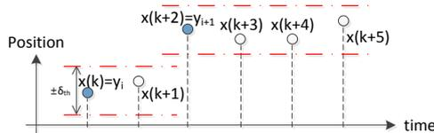
Figure 3: Reduction by deadband: If  $x(k+i)$  is within the threshold, i.e.,  $|x(k+i) - y_i| \leq \delta_{th}$ , it will be abandoned, otherwise, it will set as new transmission point  $y_{i+1}$ .
