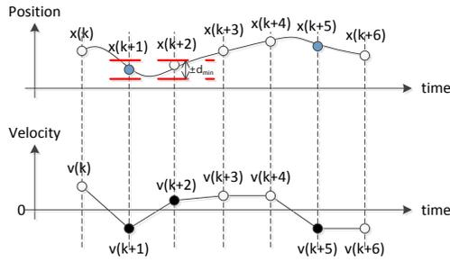
Figure 2: The anchor point is defined as a point with zero velocity but for discretized points, an approximate anchor point is obtained.
