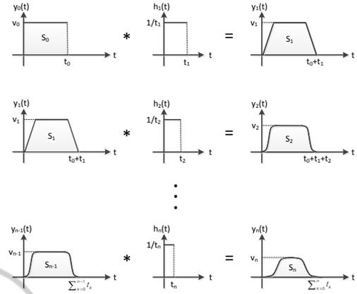
Figure 4: The effect of the convoluted trajectory with non-zero final condition is shown. The trajectory becomes smoother with more convolutions.
