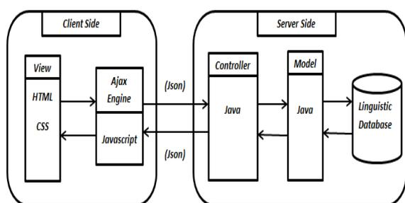
Figure 4: UKC-1 Overall Architecture.
