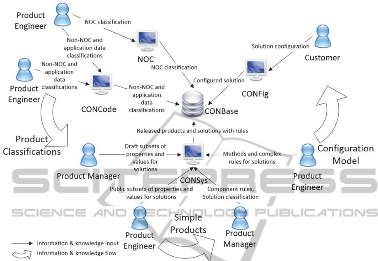
Figure 4: Integrated knowledge-based workflow.
