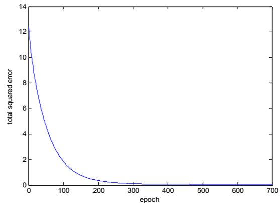
Figure 2: The total squared error plot of the HFD solution for the diffusion equation.
