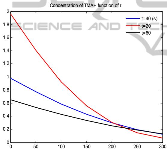
Figure 4: The Diffusion of TMA<sup>+</sup> at different times.
