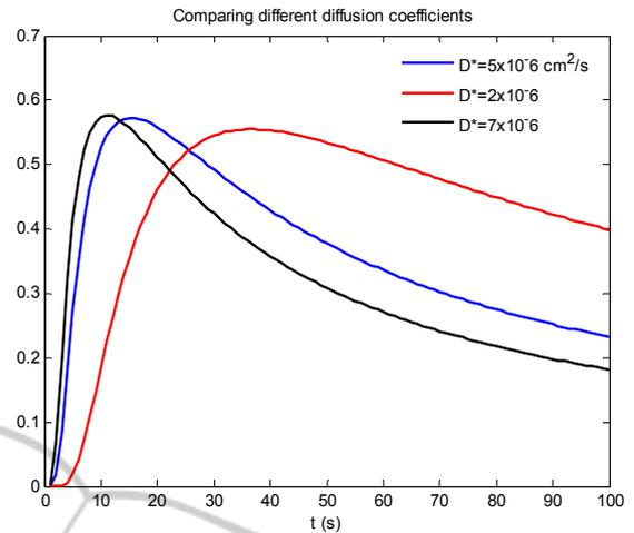
Figure 6: The concentration of TMA<sup>+</sup> with different Diffusion coefficients.
