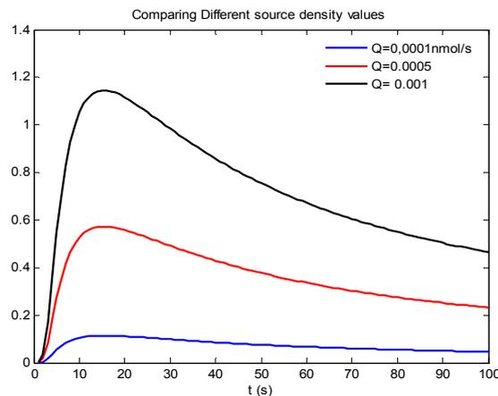
Figure 5: The concentration of TMA<sup>+</sup> at different source density values.
