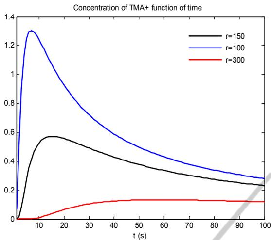
Figure 3: The diffusion of TMA<sup>+</sup> at different radial distances.
