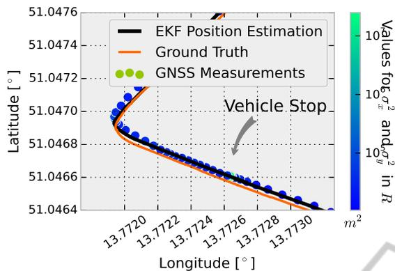
Figure 11: Detailed view of the stop within the performed test drive with raised uncertainty for  $R$ . (GNSS measurement dots are reduced to every 10th for better visualisation in this figure).
