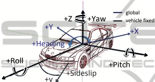
Figure 2: Right hand coordinate system with z-axis to top.
