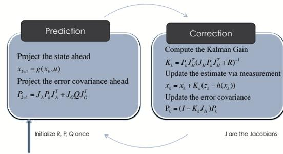
Figure 1: Extended Kalman Filter Step.
