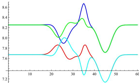
Figure 3: Module forces  $|F_i|$  in the four ropes during the maneuver, including simultaneous wind gusts along the  $\{x, y, z\}$  axes.
