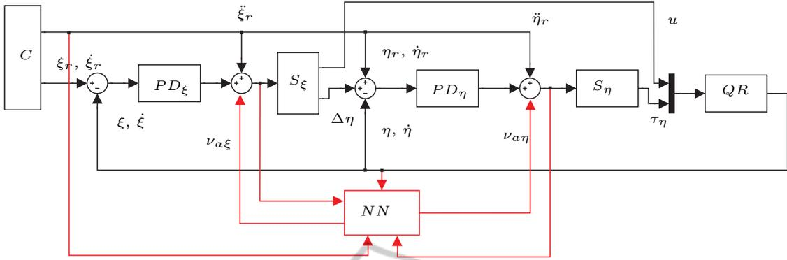
Figure 2: Augmented Linear Controller with an Adaptive SHL-NN.
