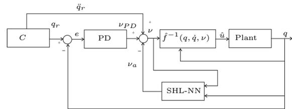
Figure 7: NN augmented adaptive control architecture.
