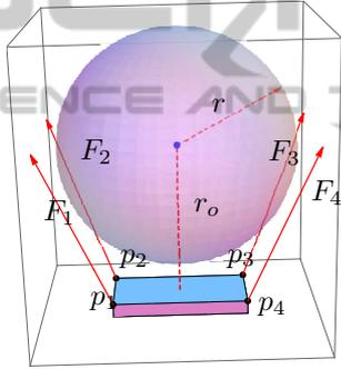
Figure 1: Auxiliary sphere in the definition of feasible lifting forces.
