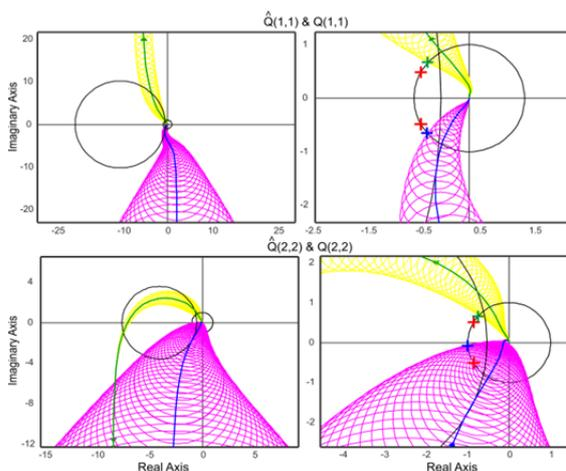
Figure 4: Nyquist-array of the designed loops.
