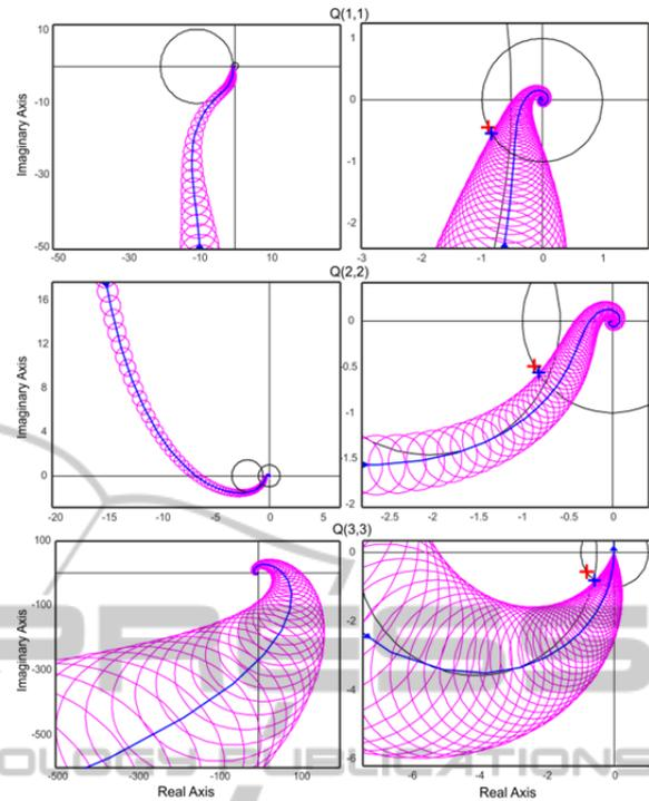
Figure 5: Nyquist-array of the designed loops.
