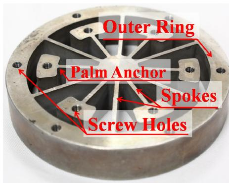
Figure 4: Photograph of Orange-slice-alike flexible body.
