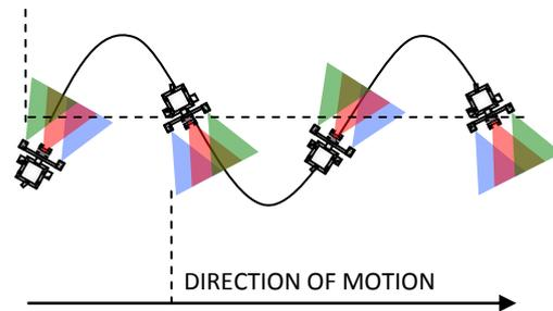
Figure 2: The visible range of sensors in a sinusoidal movement.
