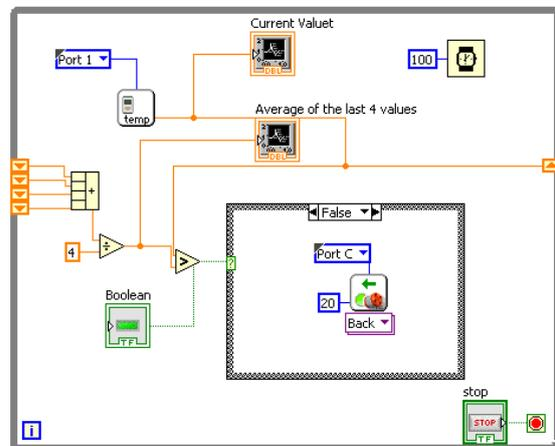
Figure 6: Single sensor based increasing gradient tracking in LabVIEW implementation.
