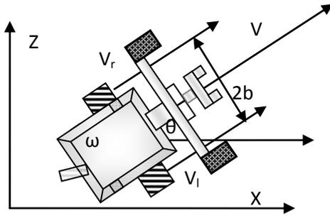
Figure 1: Differentially driven mobile robot.
