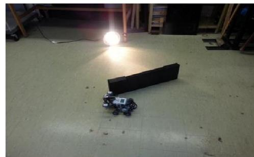
Figure 9: Robot starting behind an obstacle and moving on a sinusoidal path while detecting the heat source.
