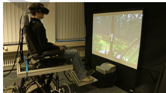
Figure 12: An advanced user interaction device. The user is wearing a VR helmet, the screen is solely for spectators.
