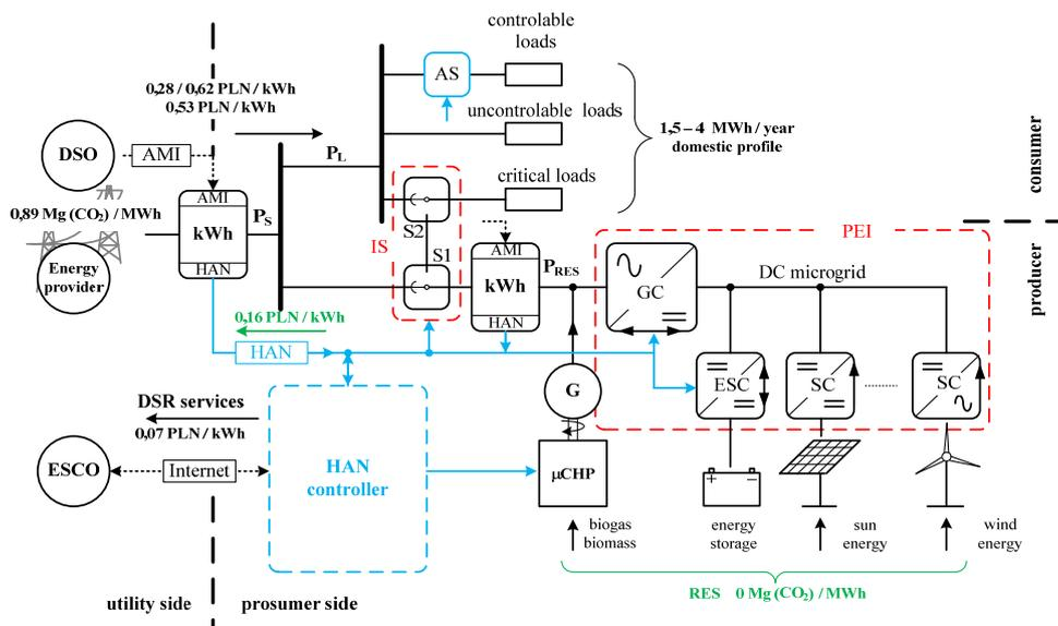
Figure 1: Unified and simplified schema of prosumer system with energy management technologies.
