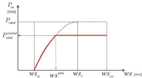
Figure 6: Normal/Restricted Output Characteristic of WT.
