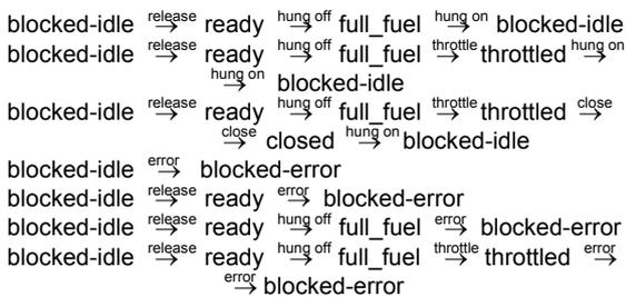
The states full\_fuel and throttled appear to be hazardous from the viewpoint of unchecked flow because the motor is on and the liquid is under pressure -- the only nozzle valve controls an issue in
