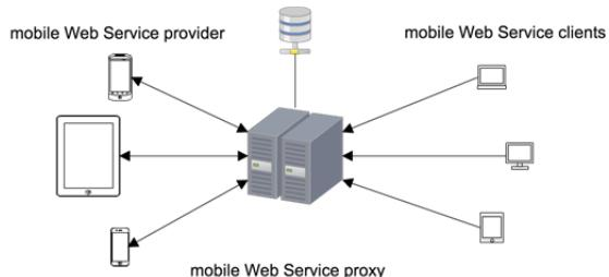
Figure 3: Architecture for providing synchronous mobile Web Services.
