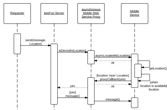
Figure 6: Location-based messaging flow using the asynchronous mobile Web Service approach.
