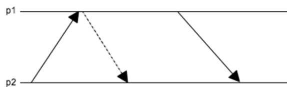
Figure 2: An asynchronous service request between a service provider (p1) and a service consumer (p2).
